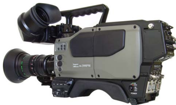
A special version of TA1520 docked with an Ikegami HK-399PW camera head.
